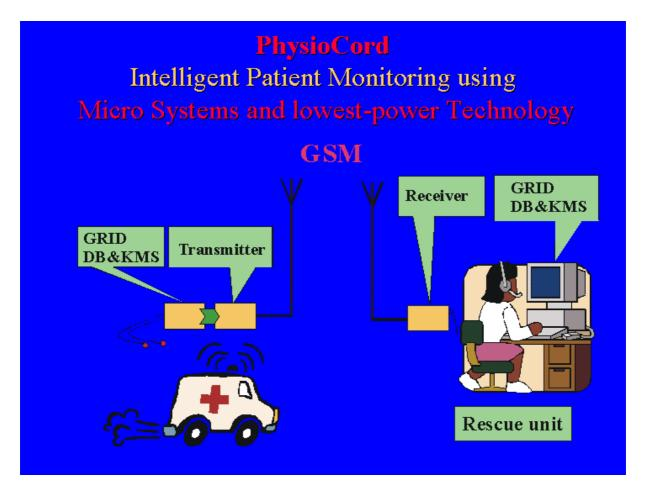
The progress of computer science has brought with it additional demands for the integration of various technologies onto the portable computer and at the same time has given rise to many novel applications. In the application presented here, the minimized portable **PhysioCord** is used with a standardized interface connecting the amplifier for ECG and other signals. Wireless data transmission is used.
