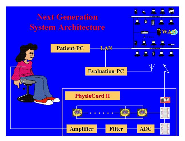
The next Generation System Architecture is characterised by high performance portables. The portable is integrated by wireless data transmission technology for the direct communication in risk situations with high data transmission rates. The high performance stationary system with DB & KMS supports the physician by the evaluation of the incoming signals in risk situations.
